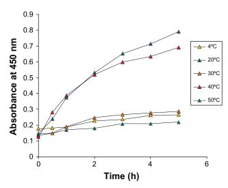
**Figure 4** Time course of silver nanoparticles formation obtained with 1 mM AgNO<sub>3</sub> using *Dioscorea bulbifera* tuber extract with different reaction temperatures.
