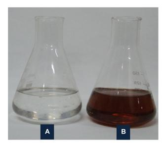
**Figure I** Solution of I mM AgNO $_3$  (**A**) before and (**B**) after bioreduction by *Dioscorea bulbifera* tuber extract at 40°C.
