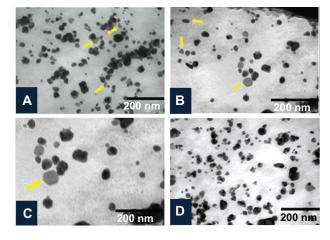
**Figure 5** Characterization of silver nanoparticles formed with 1 mM AgNO $_3$  and 5% *Dioscorea bulbifera* tuber extract at 40°C by transmission electron microscopy. (**A**) Silver nanotriangles and nanorods, (**B**) anisotropic silver nanoparticles, (**C**), silver nanohexagon, and (**D**) irregular silver nanoparticles.
