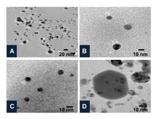
**Figure 6** Characterization of silver nanoparticles formed with 1 mM AgNO $_3$  and 5% *Dioscorea bulbifera* tuber extract at 40°C by high-resolution transmission electron microscopy. (**A**) Silver nanoparticles at a resolution of 20 nm, (**B** and **C**) spherical silver nanoparticles, and (**D**) Hexagonal silver nanoparticles.
