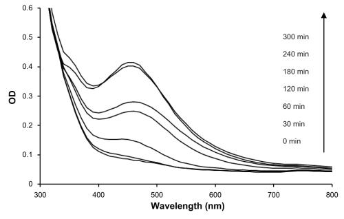
Figure 2 Ultraviolet-visible spectra recorded as a function of reaction time of I mM AgNO<sub>3</sub> solution with Dioscorea bulbifera tuber extract at 40°C.
